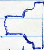
section through Lamb's tongue mould
